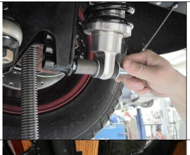
You can now install the coil-overs using the provided 5/8" hardware. The threaded side goes down as per the picture.
