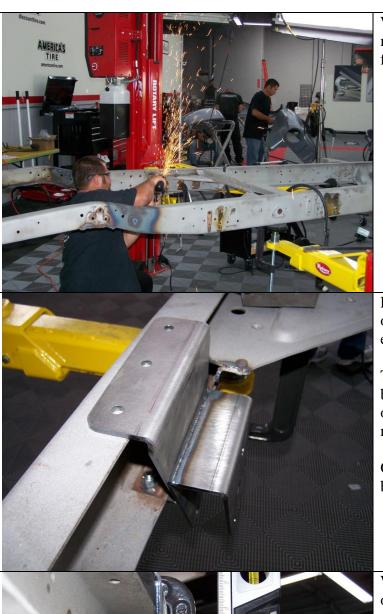
We used an angle grinder to remove this part of the cross member. Just trim it back until the existing holes on the frame line up with the bracket.
